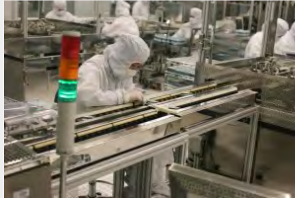
Figure 4.19 Assembly of notebook hard drives in Seagate's "clean room," Wuxi China. (Photo courtesy of Robert Scoble/Flickr.) CC BY 2.0
